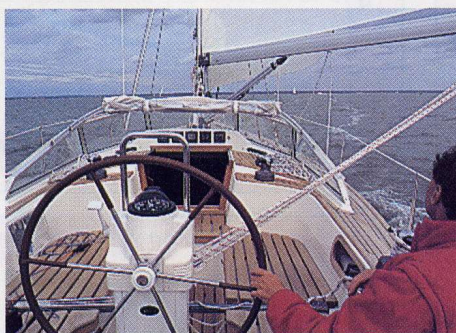
Above, the high cockpit coamings are wide enough to provide comfortable seating and good visibility downwind. Left, upwind under full sail in 14-18 knots
